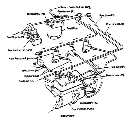
4. Using the 5/16" box wrench or the 1/4" drive 5/16" socket wrench, open the #3 bleed screw and bleed this portion of the fuel injection pump in the same manner as described in step #3. Proceed to step #5
