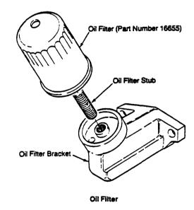
filter gasket's sealing surface on the engine block free of oil and apply a thin coat of clean engine oil to the rubber gasket on the oil filter. Screw the filter onto the threaded oil filter stub, and then tighten the filter firmly by hand. See the "TORQUE SPECIFICATIONS" section of this manual for the proper oil filter tightening specification, page 61.
