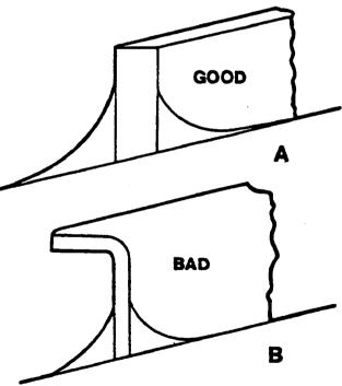
Note: Avoid excessive height, use solid stringer construction (A).
