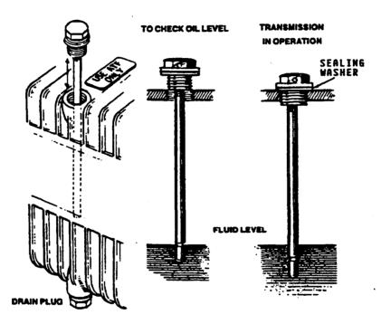
The Transmission drain plug is located directly below the dipstick and is the same size hex head as the dipstick. This drain plug also has a sealing washer.
