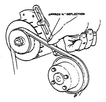
Alternator and Water Pump Belt Tension
