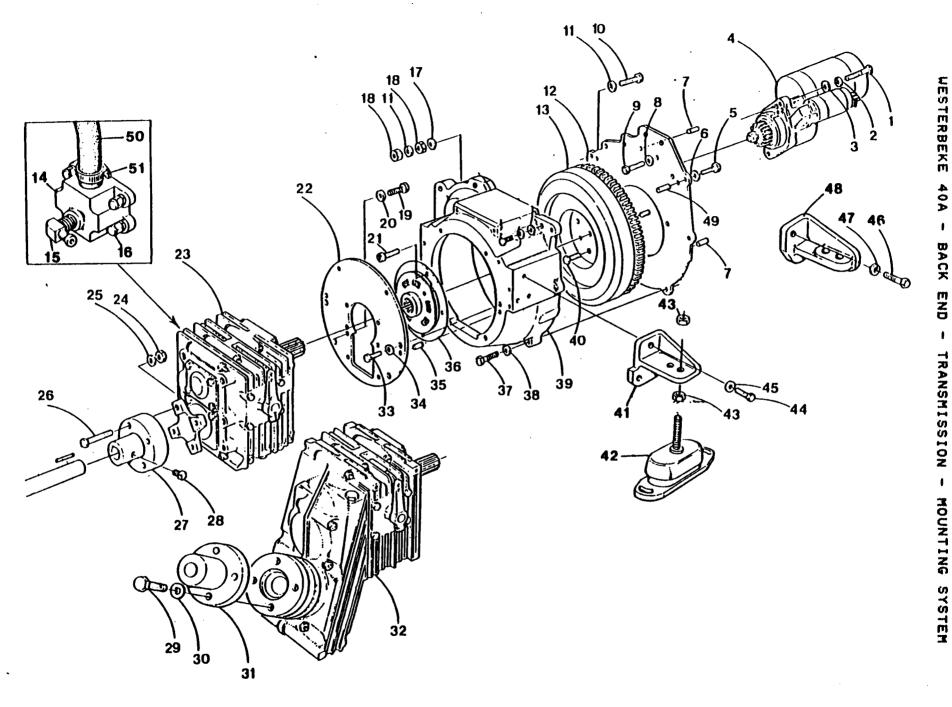
I BACK END ł TRANSMISSION I MOUNTING SYSTEM WESTERBEKE 40A - BACK END - TRANSMISSION - MOUNTING SYSTEM
