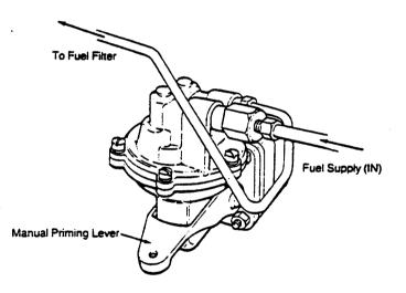
Mechanical Fuel Lift Pump
