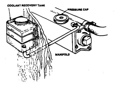
Coolant Recovery Tank, Recommended Installation
